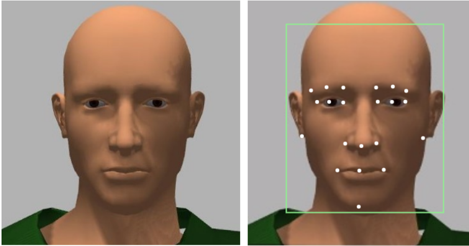
Fig. 3.11 Image of actor model taken by one of the RGB cameras with facial features detected by the CASIR attention middleware (note: in this preliminary test, the image was captured and processed while the actor was stationary).
