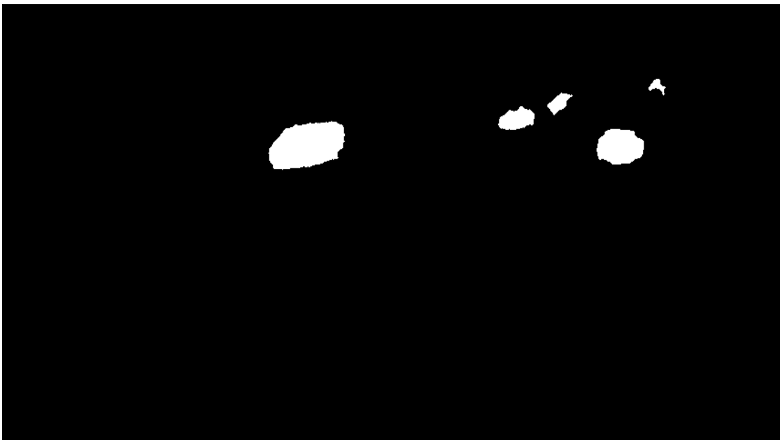
Fig. 4.5: Example of the shadow elimination applied to Figure 4.1 frame. Foreground pixels in white, background pixels in black.
