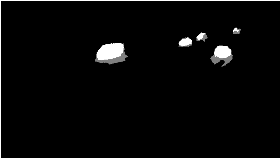
Fig. 4.4: Example of the described background subtraction algorithm with shadow detection applied to Figure 4.1 frame. Shadow pixels in grey, foreground pixels in white, and background pixels in black.
