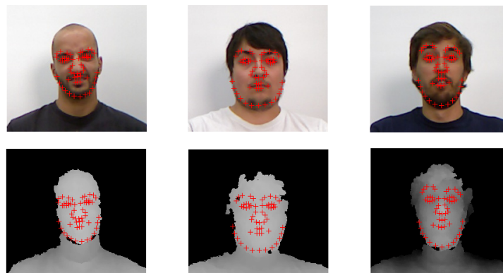
Fig. 6.5: Some marked faces from the created Database with the corresponding depth image
