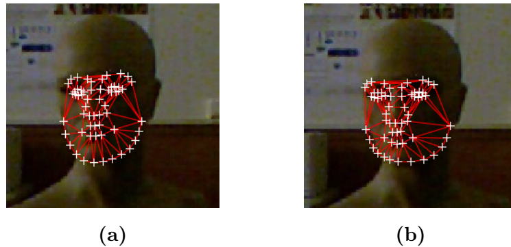
Fig. 6.7: Fitting Process in poor lightning conditions. Figure 6.7a is the fitting with HOG while Figure 6.7b represents the fitting with HOG+HONV
