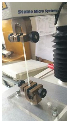
Figure 21. Visual observation of a tensile test performed in a 50/50 sample, near to the fracture strain.
