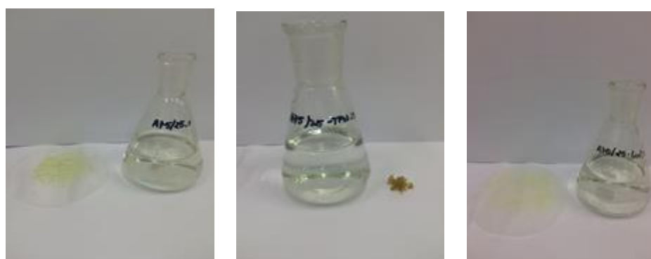
Figure 24. Visual observation of the K 2 CrO 4 solutions and of the samples 75/25 dried (left), 75/25-Tf 2 N dried (middle) and 75/25 freeze dried (right) after the experiment.
