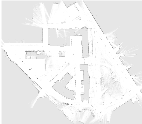
Figure 2.7: Example of a map generated with gmapping - map of the Freiburg Campus [15].
