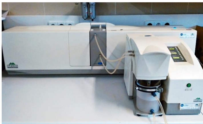
Figura 11 - Mastersizer 2000E com Hydro 2000MU.
