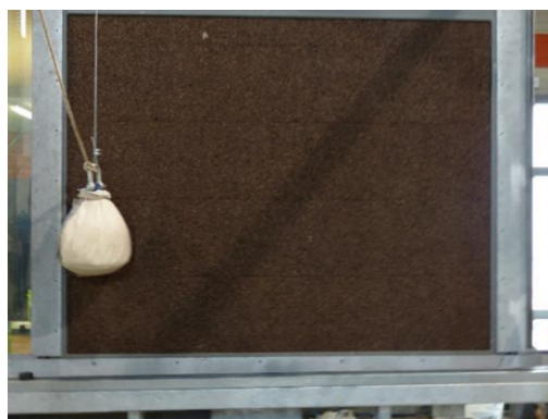
Figure 6-13: Soft large body impact test.
