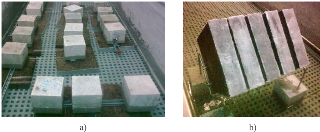
Figure 3-11: Test specimens: a) During immersion; b) Draining stage.
