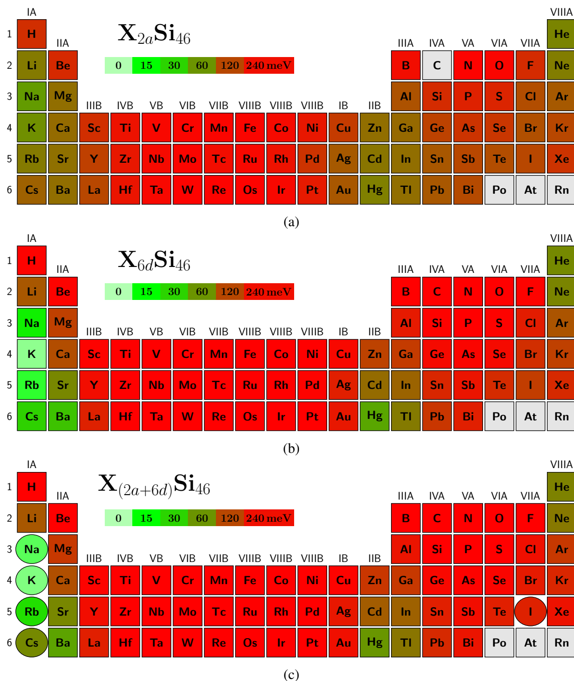
Figure 4.3 Distance to the convex hull (in meV per atom) for the clathrate X_{2a}Si_{46} (a), X_{6d}Si_{46} (b), and X_{2a+6d}Si_{46} (c). The circles denote phases with similar stoichiometries that were synthesized experimentally: X_8Si_{46} ( X=Na, K, Rb, Cs, I ) [142–145]
