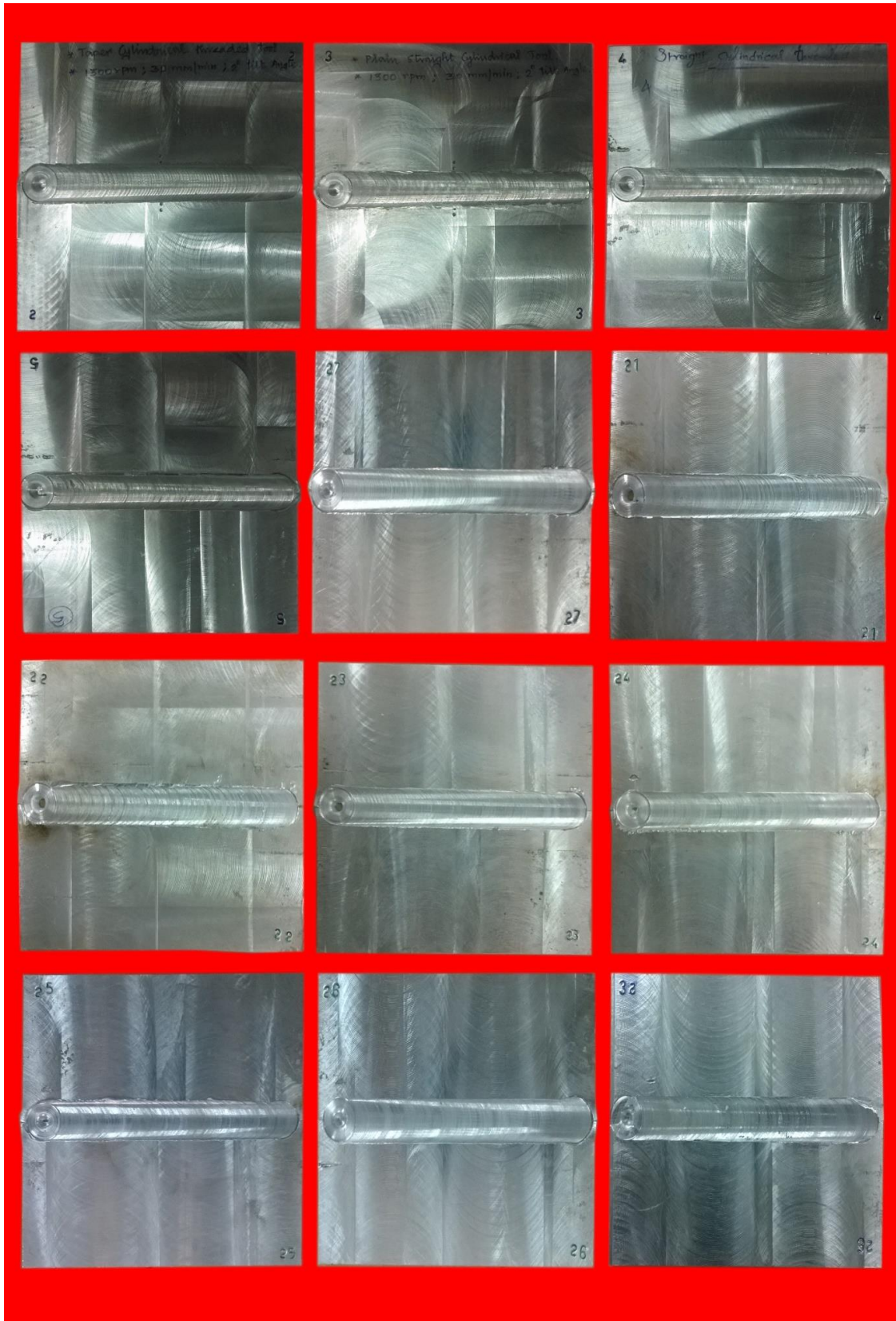
Fig. 3.6 Photograph of fabricated FSW joints
