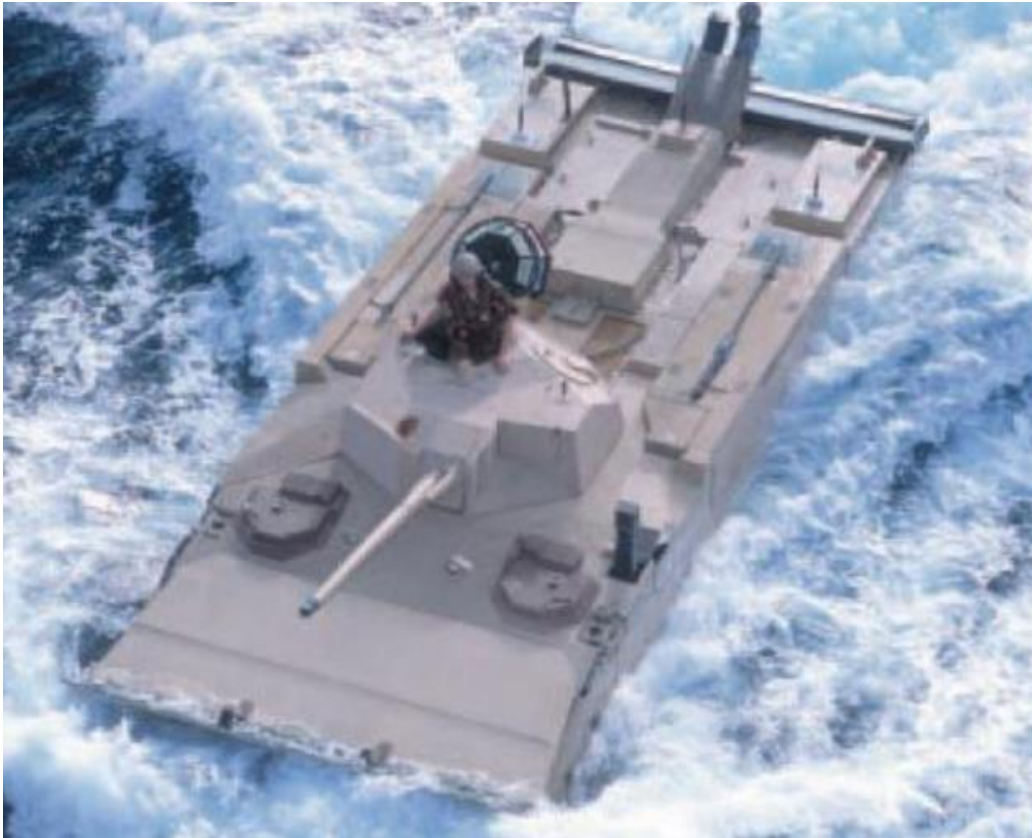
Fig. 1.3 Expeditionary Fighting Vehicle (EFV) having 2519 structure (Cho and Bes 2006)
