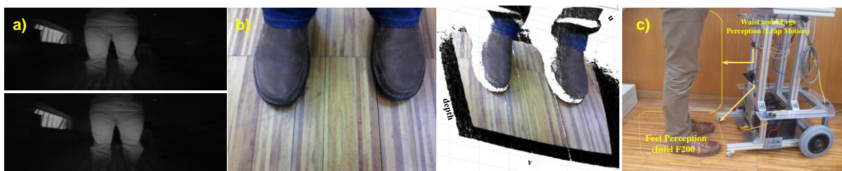
Figure 3.3. Raw data of the sensors and multimodal setup on board the ISR-AIWALKER: a) raw IR images of the Leap Motion sensor, b) shows on the left the RGB image and on the right the colored depth map, and c) presents the multimodal setup on board the ISR-AIWALKER and the sensors' regions of interest.
