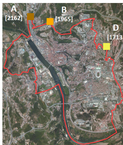
Figure 2.11: Optimum locations for three park-and-ride facilities in the municipality of Coimbra (figures in brackets represent the number of trips intercepted by each facility).
