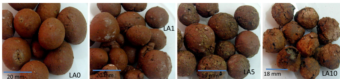
Fig. 8. Lightweight aggregates for 0, 1, 5 and 10% of incorporation.
