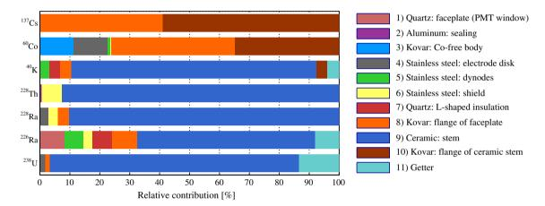
**Fig. 5** Contribution of individual raw materials of the R11410-21 phototube to the total contamination in <sup>238</sup>U, <sup>226</sup>Ra, <sup>228</sup>Ra, <sup>228</sup>Ra, <sup>228</sup>Th, <sup>40</sup>K, <sup>60</sup>Co and <sup>137</sup>Cs. The component *numbers* correspond to those in Fig. 1 and Table 2
