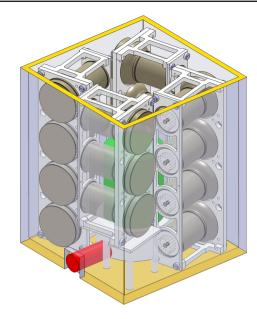
**Fig. 3** Schematic view of 15 R11410-21 PMTs in the Gator detector chamber, held by custom-made, low-background PTFE support structure. The germanium detector in its cryostat is seen in *green* in the centre
