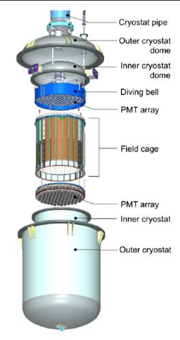
Fig. 2 The XENON1T TPC with cryostat, subgroups are indicated with reference to the "XENON1T Use" column of Table 1
