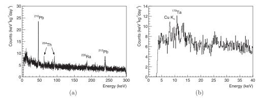
**Figure 1.** Background spectrum of the detector Ch47. The visible  $\gamma$ -lines originate from external radioactivity and cosmogenic activation. Panel (b) shows a zoom to the low-energy region.
