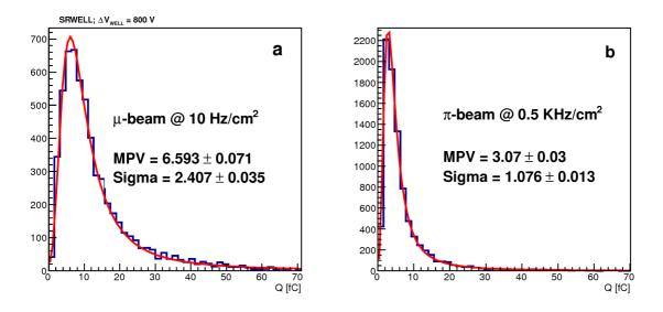
**Figure 8**. Cluster charge distributions measured with the *Single2* configuration (table 1) at an operation voltage  $\Delta V_{SRWELL} = 800 \text{ V}$  (a) muons,  $10-20 \frac{\text{Hz}}{\text{cm}^2}$ ; (b) pions,  $0.5 \frac{\text{kHz}}{\text{cm}^2}$ . The measured data (blue histograms) are fitted to Landau distributions.
