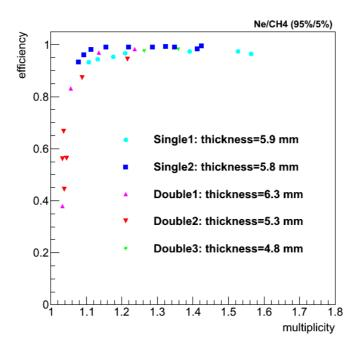
**Figure 6**. Detection efficiency with muons as a function of the pad multiplicity measured with the single-SRWELL and the double THGEM+SRWELL configurations listed in table 1. The total detector thickness, excluding readout electronics, is provided for each case in the figure. The optimal voltages and resulting efficiency, multiplicity and gain values are given in table 2.
