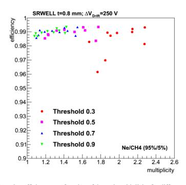
**Figure 4**. Global detection efficiency as a function of the pad-multiplicity for different charge thresholds set in the analysis, as measured with a 0.8 thick SRWELL (figure 2a) with muons. Ne/5% CH4;  $\Delta V_{\text{Drift}} = 250 \text{ V}$ .
