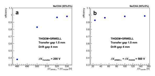
**Figure 5**. The detection efficiency with muons of the THGEM+SRWELL in a *Double1* configuration (figure 2b; table 1) as a function of applied potential. (a) Efficiency as a function of the voltage across both multipliers ( $\Delta V_{SRWELL} = \Delta V_{THGEM}$ ) at constnt  $\Delta V_{Transfer} = 200 \text{ V}$ ; (b) efficiency as a function of the  $\Delta V_{Transfer}$  at constant  $\Delta V_{SRWELL} = \Delta V_{THGEM} = 560 \text{ V}$ .
