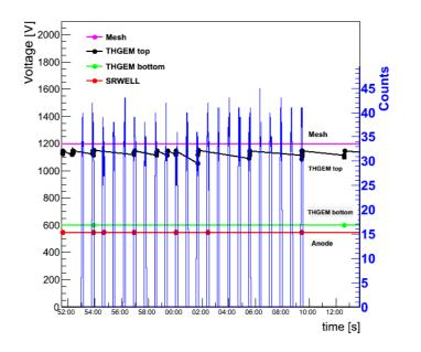
**Figure 10**. The *Double3* THGEM+SRWELL detector configuration. High-voltage variation in time overlaid on the spill structure, as measured in a pion beam at a rate of  $3 \frac{\text{kHz}}{\text{cm}^2}$ . No high voltage variations were measured on the mesh (magenta curve). The small variations (shown as dots) measured on the THGEM top electrode, THGEM bottom electrode and WELL electrode are shown in black, green and red curves respectively.
