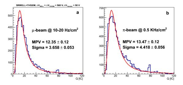
**Figure 9.** Cluster charge distributions measured with the *Double1* configuration (table 1) at operation voltages  $\Delta V_{SRWELL} = 560 \text{ V}$ ,  $\Delta V_{THGEM} = 560 \text{ V}$  and  $\Delta V_{Transfer} = 50 \text{ V}$ . (a) Muons,  $10-20 \frac{\text{Hz}}{\text{cm}^2}$ ; (b) pions,  $0.5 \frac{\text{Hz}}{\text{cm}^2}$ . The measured data (blue histograms) are fitted to Landau distributions.
