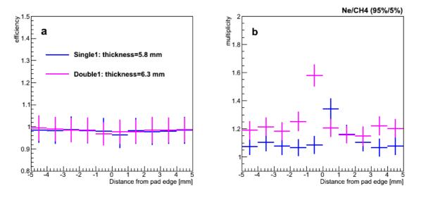
**Figure 7**. Local efficiency and multiplicity data measured with the Single2 SRWELL and the Double1 THGEM+SRWELL, using the tracking system. (a) Detection efficiency as a function of distance from the edge of the pad. (b) Pad multiplicity as a function of distance from the edge of the pad. The operation potentials are depicted in table 2.
