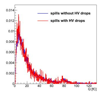
**Figure 11**. Cluster charge distributions recorded in the *Double3* THGEM+SRWELL detector (of figure 10) with pions at a rate of  $3 \frac{\text{kHz}}{\text{cm}^2}$ . The distributions were measured during spills with (red) and without (blue) micro-discharges in the same operation conditions:  $\Delta V_{\text{SRWELL}} = 550 \text{ V}$ ,  $\Delta V_{\text{THGEM}} = 550 \text{ V}$  and  $\Delta V_{\text{Transfer}} = 50 \text{ V}$  resulting in an effective gain of ~ 2500.
