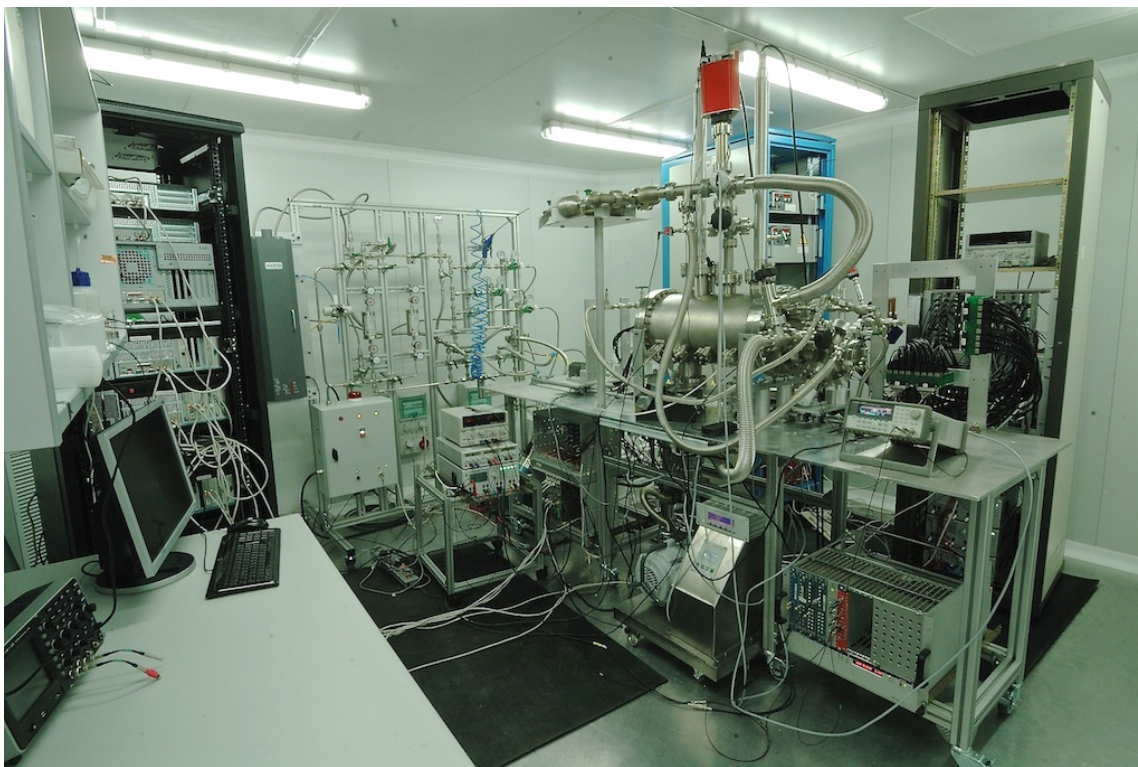
Figure 3. The NEXT-DEMO detector and ancillary systems (gas system, front-end electronics and DAQ) in their location at a semi-clean room at IFIC.
