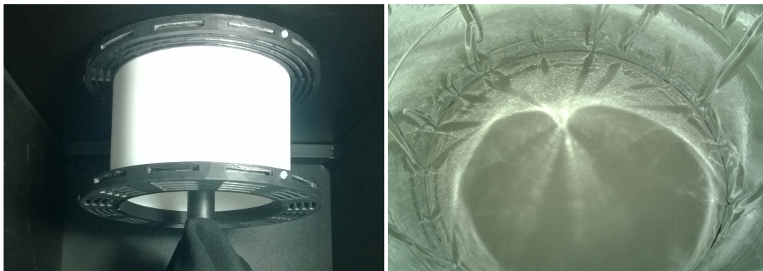
FIGURE 4.12: Left: A PTFE wall mounted on the workbench. Right: aluminized Mylar wall.
