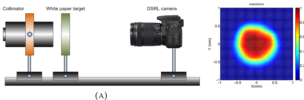
FIGURE 5.10: Left: Experimental set-up. Right: Color coded image of the measured light beam profile.
