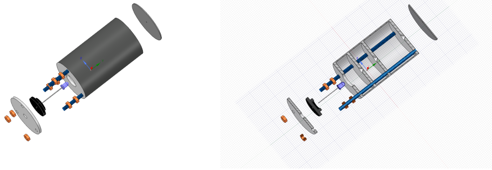
FIGURE 5.9: Collimated light source assembly: exploded view (left) and cut-away exploded view (right).
