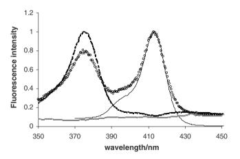
**Figure 3.** Normalised excitation spectra of H<sub>4</sub>DTPP in acetonitrile collected at different emission wavelengths: 712 nm (black thin line); 610 nm ( $\circ \circ \circ$ ); 540 nm (---) and (grey bold line for TPP-CONHBu1).
