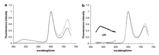
**Figure 2.** Normalised fluorescence spectra of  $H_4DTPP$  (black line) and of TPP-CONHBu1 (grey line) in acetonitrile obtained upon excitation at (a) 375 nm and at (b) 508 nm (inset: amplification of fluorescence intensity in the high energy region).
