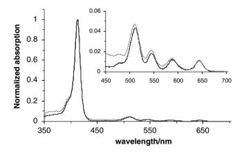
Figure 1. Normalised UV–vis absorption spectra of  $H_4DTPP$  (black line) and TPP-CONHBu1 (grey line) in acetonitrile. Inset: Expanded absorption spectra in Q-band region.
