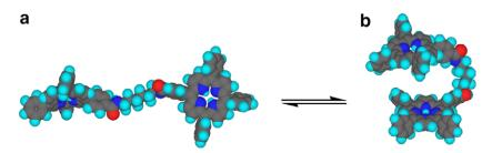
Scheme 2. Minimised conformational structures from molecular mechanical calculations (MM2) (a) 'open form' and (b) 'closed form'.
