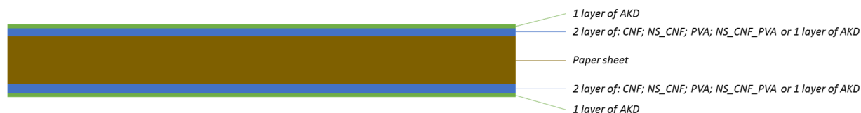
167 168 Figure 1. Schematic illustration of the structure of coated papers
