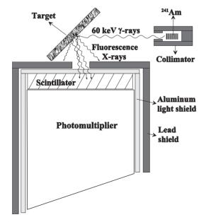
Fig. 1. Schematic of the detector and the source/target geometry.
