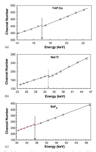
Fig. 2. Detector relative amplitude  $(\bigcirc, \Delta)$  as a function of the X-ray energy,  $E_x$ : (a) for YAP, (b) NaI(Tl) and (c) BaF<sub>2</sub> scintillators. The solid straight lines represent linear least-square fits to each set of data below  $(\bigcirc)$  and above  $(\Delta)$  the respective K-absorption edges.
