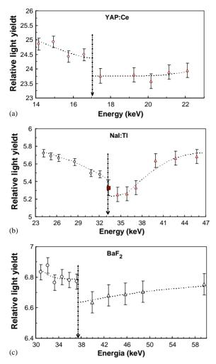
Fig. 3. Centroid channel-to- X-ray energy ratio,  $A/E_x$ ,  $(\bigcirc, \Delta)$  as a function of the X-ray energy,  $E_x$ : (a) for YAP, (b) NaI(TI), (c) BaF<sub>2</sub> scintillators, below ( $\bigcirc$ ) and above ( $\Delta$ ) the respective K-absorption edges.
