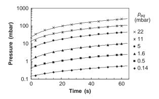
Fig. 2. Pressure evolution in the high-vacuum chamber as a function of time, after the rotary pump has been stopped, for different air leaks through the needle valve. The solid lines represent linear fittings to the different data sets.  $p_{eq}$  is the equilibrium pressure reached in the chamber while the pumping action was on.
