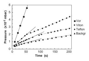
Fig. 5. Pressure rise in the high-vacuum chamber as a function of time, after the high-vacuum valve has been closed, for the different samples present inside the sample chamber. The solid and broken lines present linear fittings to the different data points in the lower and higher pressure regions, respectively.
