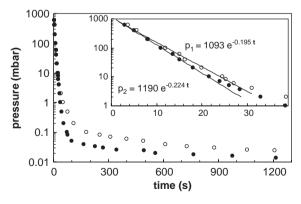
Fig. 1. Pressure evolution as a function of time in the high-vacuum chamber  $(p_1)$  ( $\bigcirc$ ) and at the rotary pump inlet  $(p_2)$  ( $\bigcirc$ ).
