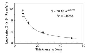
Fig. 6. Helium leak rate due to permeability through 1-cmdiameter Kapton foils as a function of their thickness for 1 bar helium pressure differential. The solid line is the best fit to the experimental data.
