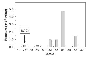
Fig. 7. Typical RGA partial pressure measurement in the mass range of 77–87 amu for a krypton leak introduced in the vacuum chamber.
