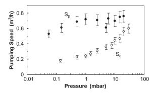
Fig. 3. Rotary pump pumping speed as a function of pressure at pump inlet  $(S_p)$  and in the high-vacuum chamber  $(S_c)$ .
