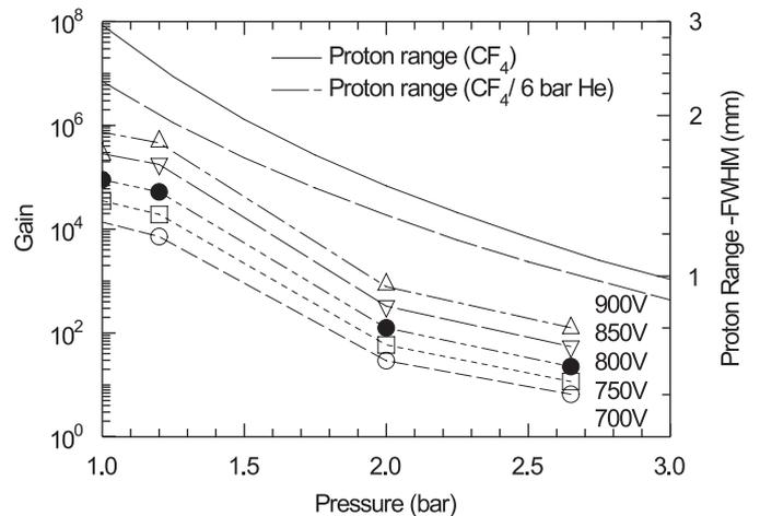
Fig. 2. Variation of MHSP gain and calculated position resolution (for  $573\ \text{keV}$  protons) with applied  $\text{CF}_4$  pressure for a number of different applied voltages. Note the additional curve showing the expected position resolution if 6 bar helium is added to a given  $\text{CF}_4$  pressure.
