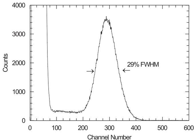
Fig. 4. Pulse height Spectrum of Mn K X-ray line (5.9 keV) from Fe-55 source with  $\text{CF}_4$  at 1 bar. MHSP was held at gain of 1000 with  $V_{CT}$  and  $V_{AC}$  at 510 and 290 V, respectively.
