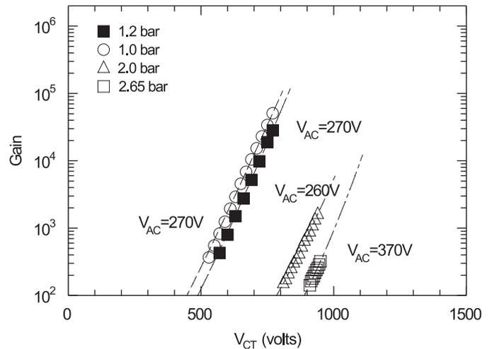
Fig. 1. Gains obtained with MHSP operating in  $\text{CF}_4$  as a function of applied voltage for a number of different pressures.  $V_{AC}$  is the voltage between anodes and cathodes on the strip-side.
