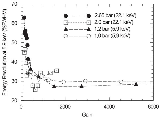
Fig. 3. X-ray energy resolution (%FWHM) of the Mn K X-rays (5.89 keV) for  $\text{CF}_4$  pressures of 1 and 1.2 bar and Ag K X-rays (22.1 keV) for  $\text{CF}_4$  pressures of 2 and 2.65 bar as a function of the MHSP gain. In all cases the drift potential  $V_T$  was maintained at 20 V.
