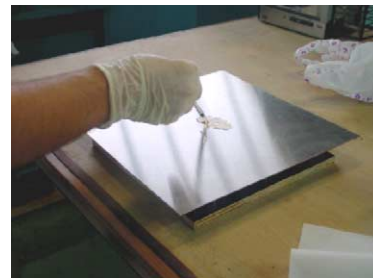
Fig. 4. Oiling blank with syringe.
