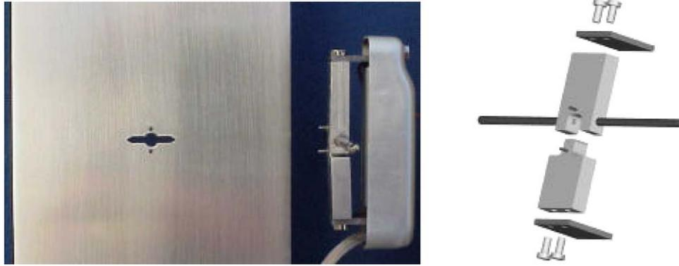
Fig. 2. Pin microgauge and corresponding position in the specimen.
