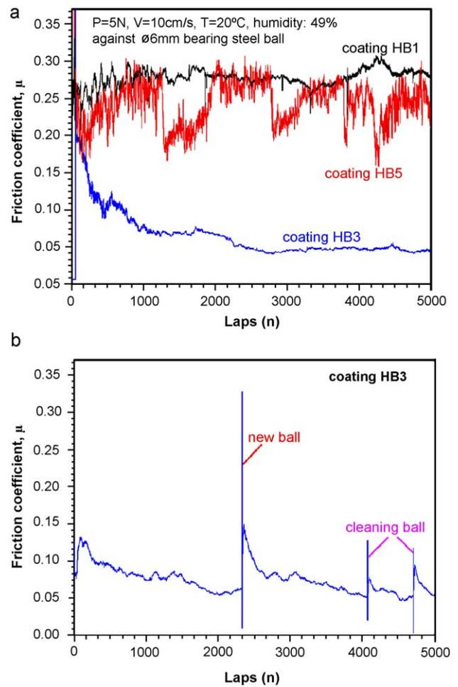
Fig. 6. Tribo-test results showing the friction coefficient of nc-TiC/a-C:H nanocomposite coatings on hardened M2 tool steel substrates: (a) three coatings against bearing steel balls and (b) self-lubrication effects observed on the coating HB3 against bearing steel ball.
