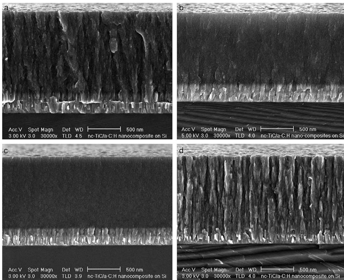
Fig. 3. SEM micrographs of fractured cross-sections showing the transition from columnar to glassy structures of nc-TiC/a-C:H coatings deposited under different conditions: (a) 110 sccm C<sub>2</sub>H<sub>2</sub> and −60 V bias; (b) 110 sccm C<sub>2</sub>H<sub>2</sub> and −100 V bias; (c) 110 sccm C<sub>2</sub>H<sub>2</sub> and −150 V bias and (d) 80 sccm C<sub>2</sub>H<sub>2</sub> and −100 V bias.
