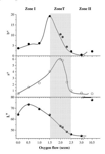
Fig. 4. Average colour coordinates in the CIELAB 1976 colour space under the standard CIE illuminant D<sub>65</sub>, for films prepared with different oxygen gas flows.
