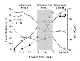
Fig. 1. Variation of the concentration of titanium, carbon and oxygen (open symbols) and the ratio  $(C_C + C_O)/C_{Ti}$  (solid circles) as a function of oxygen flow rate.
