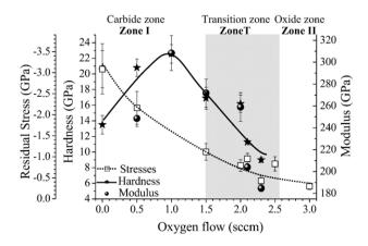
Fig. 3. Film residual stresses, hardness and Young's modulus evolution of sputtered  $TiC_xO_v$  films as a function of the oxygen gas flow.
