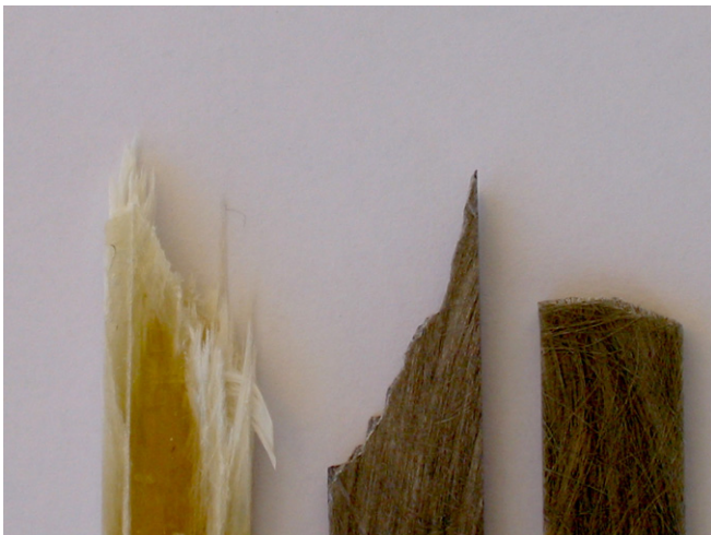
Fig. 5. Failure aspect: uncoated fibers (left); aluminized fibers stored in air (center) and immersed in water (right).
