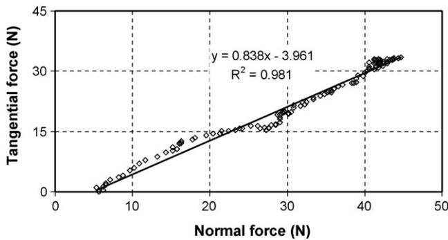
Fig. 3. Plot of the friction force against the normal load (linear, one stage). The resulting friction coefficient is the slope of the fitted linear line.
