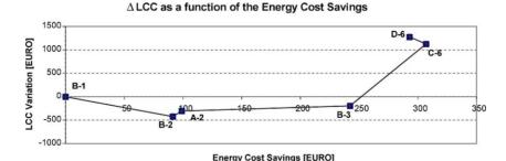
Fig. 4. Life cycle cost variation as a function of the energy cost savings, calculated in relation to the reference option (option B-1).
