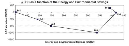
Fig. 5. Life cycle cost variation as a function of the energy and environmental cost savings, both calculated in relation to the reference option (option B-1).
