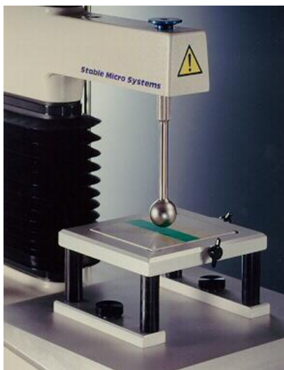
Fig. 12 Tack adhesion test with the stainless steel ball probe and double-sided tape applied on the Peltier plate.
