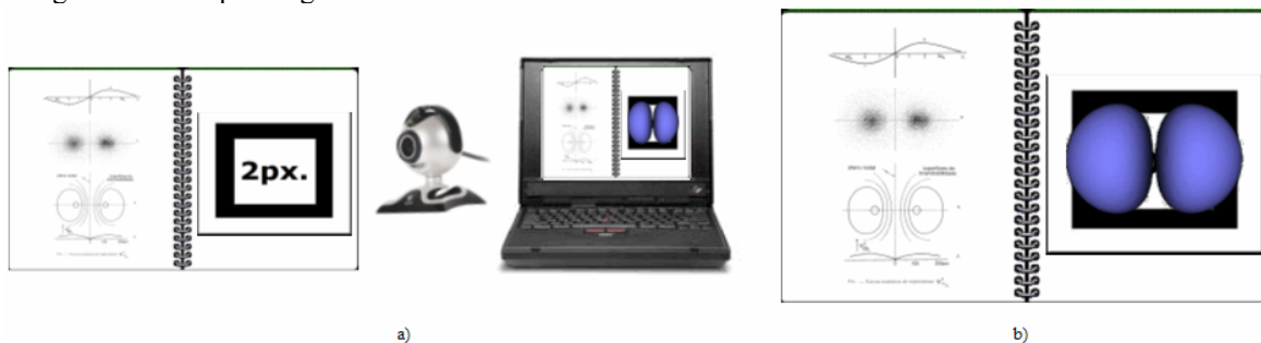
Figure 1. The representation of the 2p_x orbital through Orbitário : a) the pattern image (for example, a real image from a book) is captured by a web cam and interpreted by the software; b) the associated 2p_x orbital (a virtual model) is displayed (statically or dynamically) combined with views of a real environment
