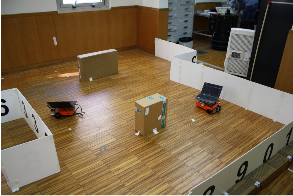
Figure 5.2: A small experiment taking place in the MRL Arena. In this experiment, a Traxbot and a Stingbot platforms were used. In this experiment, the centralized mode was used, to cope with the low processing power of the smaller laptops.
