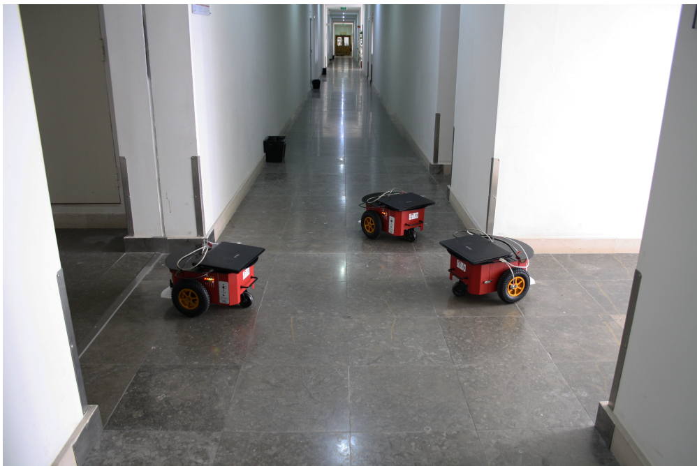
Figure 5.3: An illustration of the Institute's arrow-straight corridors, where experiments took place. In this instance, the distributed mode can be used, since the Pioneer 3-DX is able to carry larger laptops that are able to run the full system.
