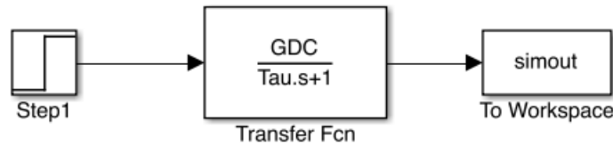
Figure 4.9: Simulink Diagram for 1st order transfer function of RobChair Storm’s Motors
