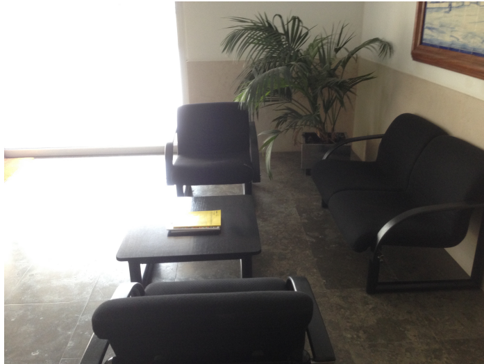
Figure 6.1: Example of a real scenario for which the 2.5D fake laser may be a problem, due to the occlusion of the table.
