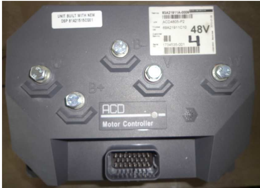
Figure 2.5: Motor Controller (ACD 4805)
