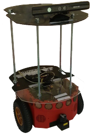
(a) Photo of the Pioneer 3-DX mobile robot the the custom structure and the Kinect on top of it.
