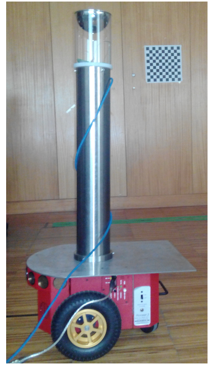
Fig. 1.1: In this figure it is presented, on the left, the True Omnidirectional system proposed by Nalwa at [26] formed by four planar mirrors and four cameras. On the right side, it is presented our system built by a non-central catadioptric imaging system and a Pioneer 3-DX robot.
