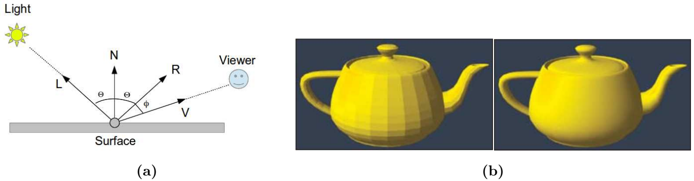
Fig. 2.3: In Fig. (a) it is illustrated the Phong reflection model (the description of the figure is done throughout the section). In Fig. (b) we show an example from [19] for the teapot object when applying different techniques of shading. On the left image a flat shading example and, on the right image, a smooth shading example (Gouraud shading).
