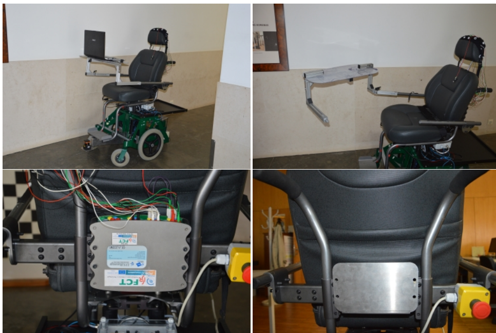
Figure 5.13: Sensor and interfaces supports added
