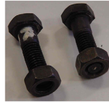
(iii) Detail of the bolts (no bending deformations).
