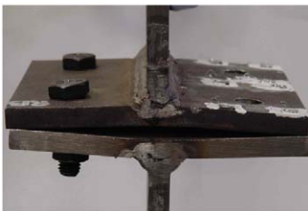
(a) Deformation at failure.
