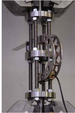
Fig. 4. Test rig for the bolt tensile testing and horseshoe device.
