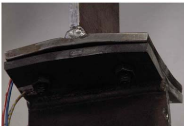
Fig. 38. Deformation of specimen WT4B at failure (two different views).
