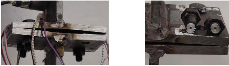
(a) Deformation at failure (WT51b). (b) Detail of a broken bolt (WT51a).
