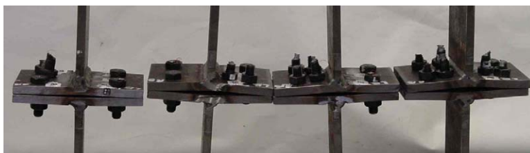
Fig. 29. Comparison of the deformation of specimens WT51, WT53C, WT53D and WT53E (from left to right) at failure.
