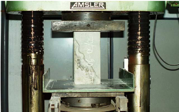
Fig. 1. Slant shear test.
