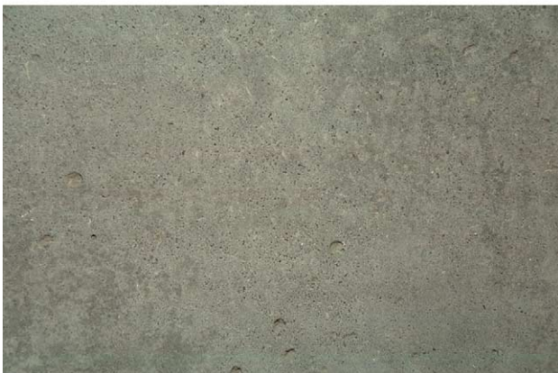
Fig. 3. Substrate surface prepared with steel brush.
