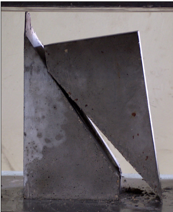
Fig. 4. Slant shear test adhesive failure.
