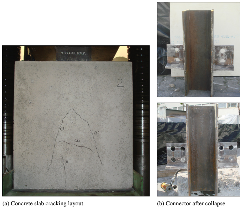
Fig. 13. T-Perfobond connector failure modes.
