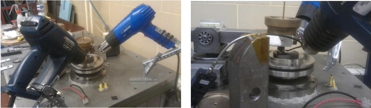
Figure 21 - Pin on disk apparatus with heating equipment
