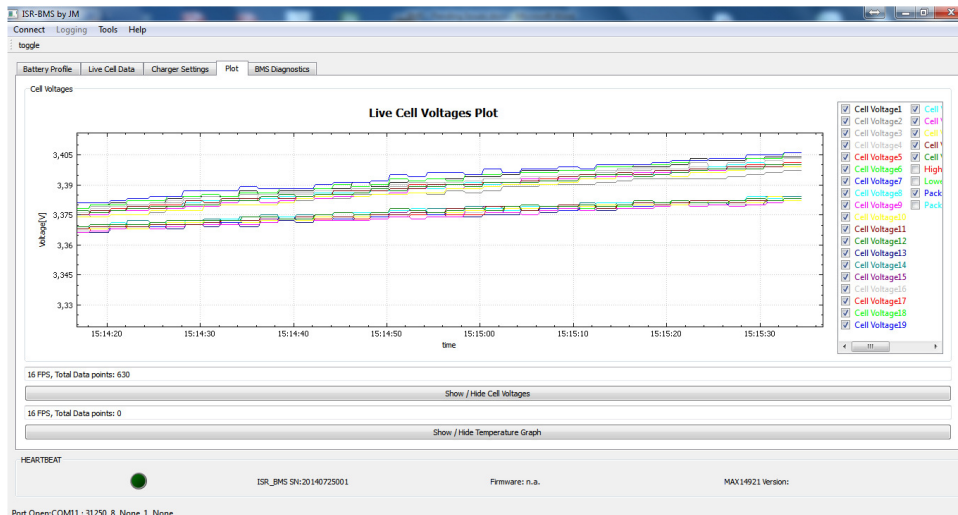
Figure 5.4: Cell voltages during charge at 10A constant current.
