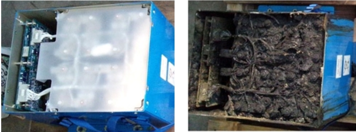
Figure 2.8: Lithium Battery from Boeing Dreamliner Airplane safety failure.
