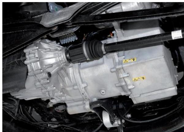
**Figura 12. Imagem do motor seleccionado [Brochura ZYTEK IDT 120-55 Integred 55 kW Electric Engine, Zytek Automotive].**
