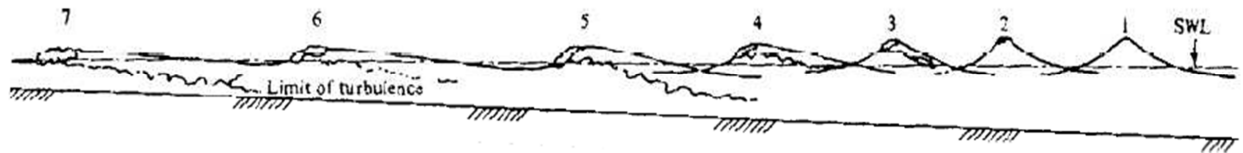
Figure 2 - Spilling wave breaking (numbers present the steps of breaking), (Source: Richardson, 1996).
