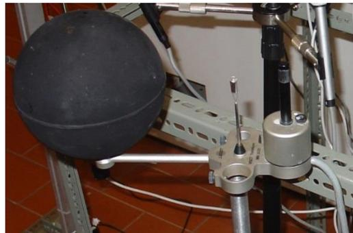
**Figure 0.9.** WBGT set of sensors (including the black globe).
