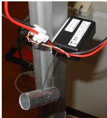
**Figure 2.4.** Thermistor with aluminium foil protection.
