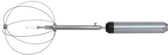
**Figure 0.7.** Swema's anemometer.
