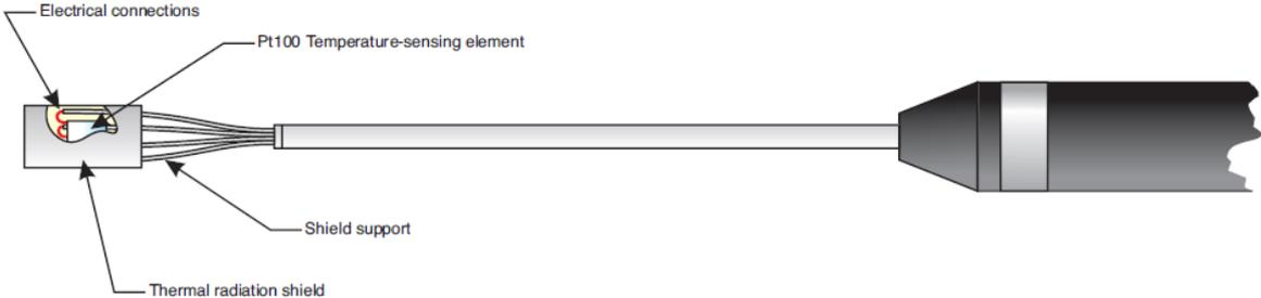
Figure 0.5. Air temperature transducer.
