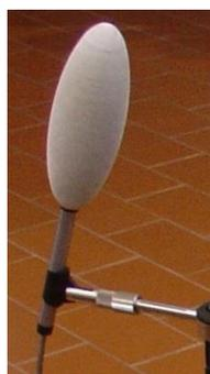
**Figure 0.8.** Thermal comfort transducer.
