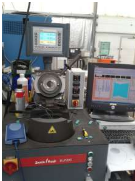
Figure 3.3 – Zwick/roell-BUP200 device and the acquisition system.
