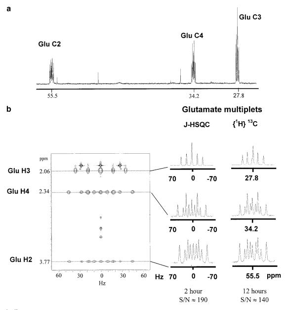
**FIG. 2.** (a)  ${}^{1}H{}^{13}C$  NMR spectrum and (b) J-HSQC spectrum collected at 14.1 T of an extract of a mouse heart perfused to steady state with a mixture of  $[2 \cdot {}^{13}C]$  acetate and  $[1,2 \cdot {}^{13}C_{2}]$  acetate. The projection of the J-HSQC and the  ${}^{1}H{}^{13}C$  spectrum give the same multiplet data. Note the loss of isotopic shift in the J-HSQC spectra.
