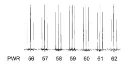
**FIG. 1.** The effect of imperfect refocusing pulses on the multiplet intensities of the 2:1  $[1,2^{-13}C_2]$ : $[2^{-13}C]$ acetate standard. The appropriate RF power was calculated to be 59 dB by the pulse-shaping software.
