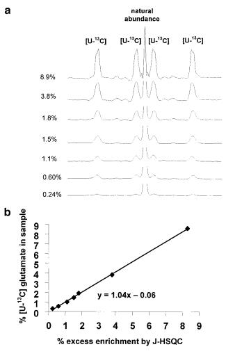
FIG. 4. (a) J-HSQC spectra of glutamate containing various amounts of added [U-13C]glutamate. Total glutamate was 150 mM. (b) Plot of known chemical excess enrichment of  $[U^{-13}C_5]$ glutamate as measured analytically versus excess enrichment as measured by J-HSQC. The latter values were obtained by measurement of quartet versus singlet resonance areas in each spectrum.
