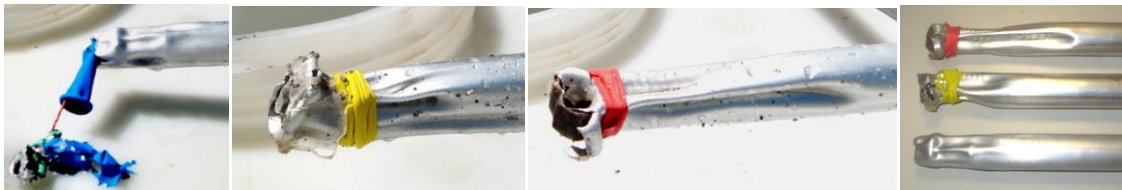
Figure 6.12. Deformed aluminium support tube, as a function of used charge ( 5 g left, 10 g center and 15 g right and their group).
