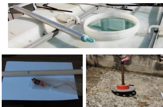
Figure 5.2. Explosive support structure for the experimental tests. On the top the alluminium tube having the small charge at the end. On the bottom the ones for the 25 lt jerry cans – on the right a plate adapter, and on the left a vertical plastic tube.
