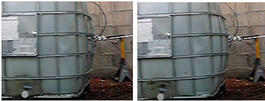
Figure 6.25. Video frames from the external deformation of plastic container on the final states before the water comes out, using 7.2 g PETN plus standard detonator as charge, inside a 1000 litres water container.
