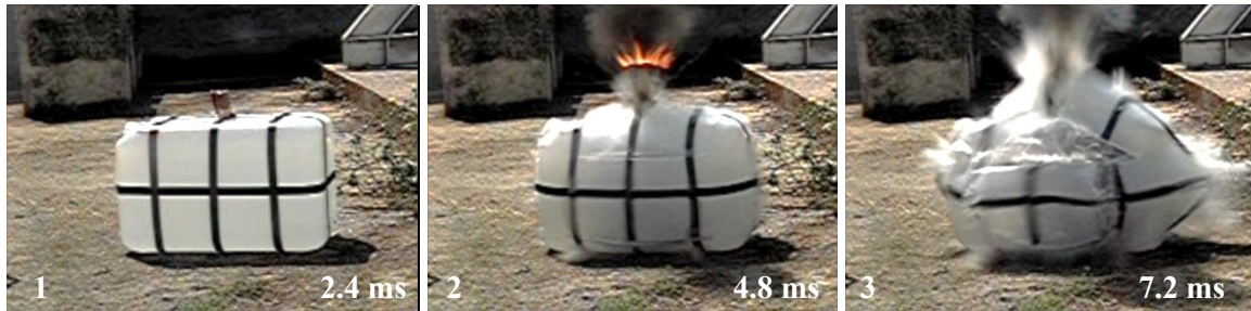
Figure 5.14. Blast type experiment – 2.4 g of PETN plus detonator No. 8 and 25L container.
