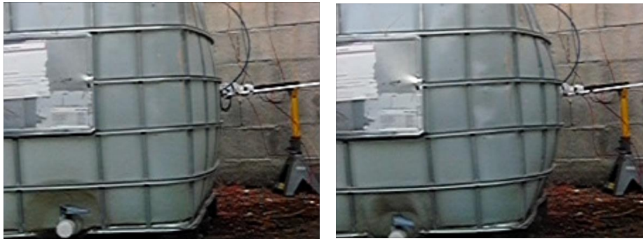
Figure 6.24. Video frames from the external deformation of plastic container on the detonation initial states, using 7.2 g PETN plus standard detonator as charge, inside a 1000 litres water container (initial point left, detonation point right).
