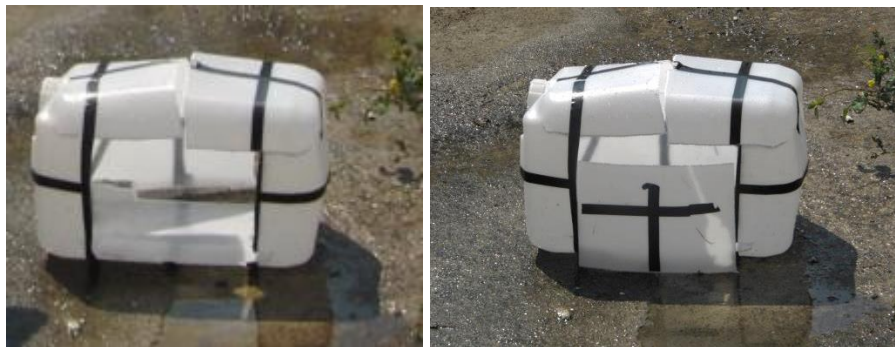
Figure 5.15. Final state of the blast type experiment – 2.4 g of PETN plus detonator No. 8 and 25L container.
