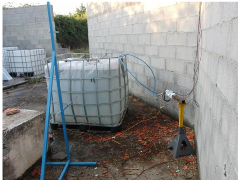
Figure 5.12. Plastic 1000 litres container, with the pressure set-up plate and the distance set-up.
