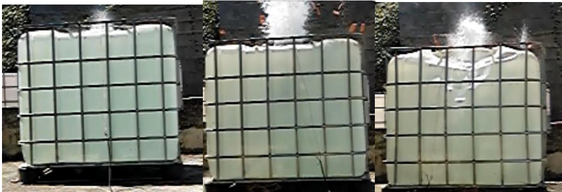
Figure 6.13. External deformation of plastic container and observed reflections for the 3 tested charges (5 g left, 10 g center and 15 g right).
