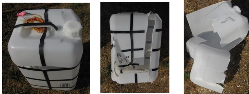
Figure 6.23. Final images of the 25 litres container – on the left the first class of tests and on the center and right the second class of the tests respectively.
